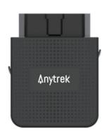
VT2216 is an intelligent OBD solution, which integrates CatM1/GPRS modem, Bluetooth, 3D Accelerometer Gyro and GPS. Developed on Qualcomm chipset, it supports different applications and is an ideal option for in-vehicle smart terminals.
