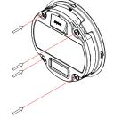
Fix the main unit with four screws provided.
