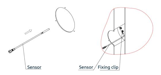
Fix the sensor with the fixing clip
