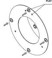
Use four rivets provided at the holes pointed by arrows.
