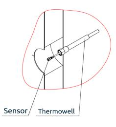
Fix the sensor with the fixing clip
