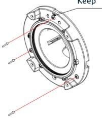
Use three rivets provided at the holes pointed by arrows.
