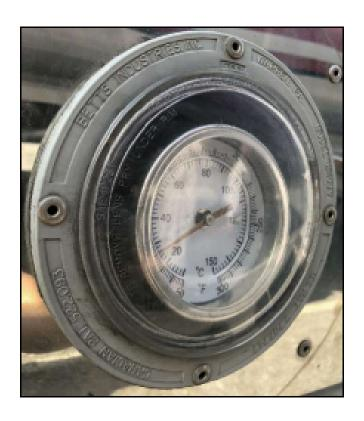
Remove thermometer and gauge holder
