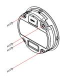
Fix the main unit with four screws provided.
